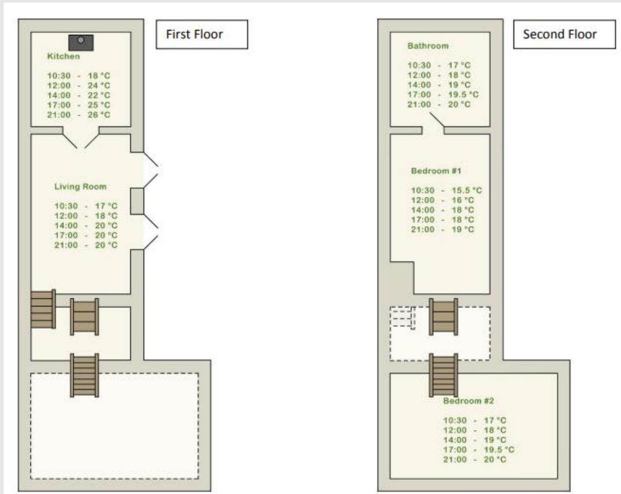
The Bathroom is the hardest area for the heat to penetrate having to pass from the kitchen, through the living room, up the stairs, through bedroom #1. The heat difference between the stove and the Bathroom (the furthest room) at 17:00 the temperature difference is only 5.5°C (about 1°C per room difference) with 6°C external temperature.
