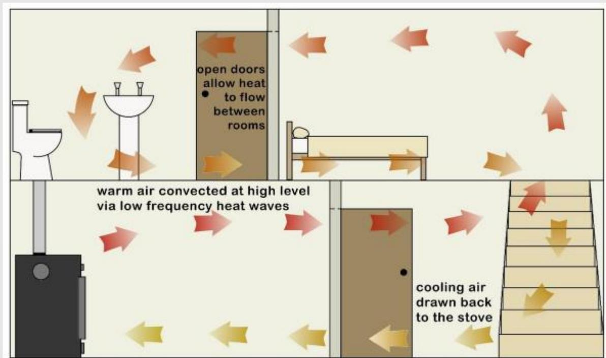
As the stove is continually heating the air the returning air is warm as opposed to cold giving a balanced temperature
